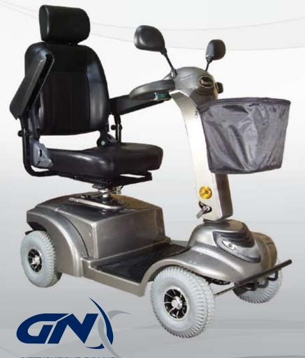
Born from the new generation of Orthoquad mobility scooters, the ES950 establishes a new bench mark for mid-size scooters. Powered by the new 950 watt 4 pole engine and coupled with two (2) 40 amp batteries, it delivers top performance with an impressive range. The ES950 has an amazing adjustable 4 wheel suspension for enhanced performance on rugged terrain.
